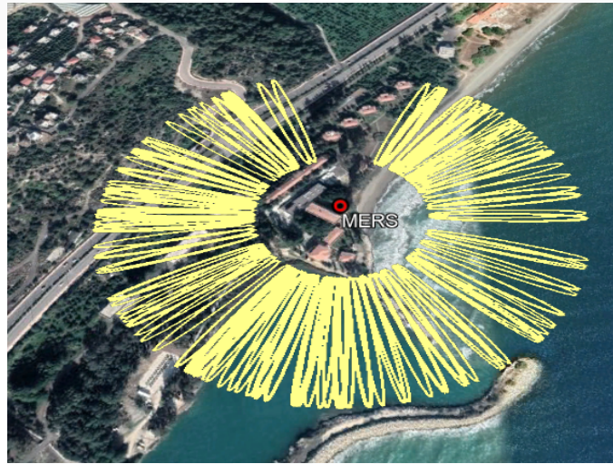
Figure 4. MERS station Fresnel zones according to satellite elevation angle of 4^{\circ} .
